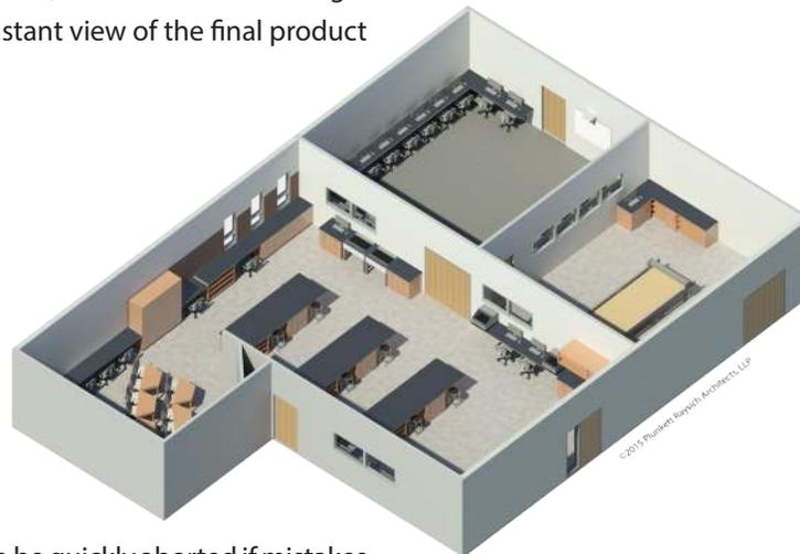
Jobs can then have the ability to be quickly aborted if mistakes are detected from inception. When installing the CNC router, it is important to build a separate enclosure to help dampen the noise generated by the machine. Being able to contain the dust and particles produced is another benefit to placing the router in an isolated room. Instruction is an essential aspect of a Fab Lab and should be defined by partitions away from both
